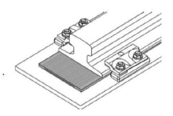
First and utmost the rail pad should conform to chosen rails. Rail pad can be used in and outdoors. Top surface of the rail should be free of oils, thick and slippery materials. They can cause rail pad damage. The pad should be placed on bearing surface gapless wavy surface up. Pads should be placed in full compliance with lower rail edges to cover top parts all over.
